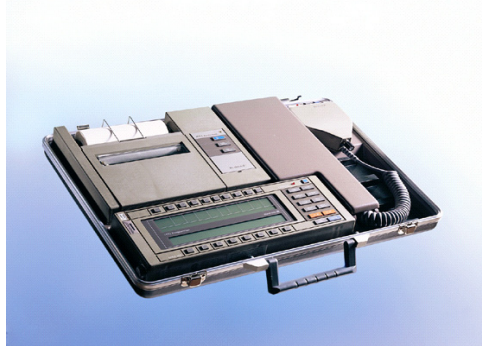
Programming equipment: handheld programmer and console programming unit used by the neurologist or specialized nurse to program the stimulators. Courtesy of Medtronic, Inc
